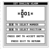
in the depth. For example, to set the shallow alarm depth to 10 feet, press the right arrow key once, then press the up arrow key once. The changes
